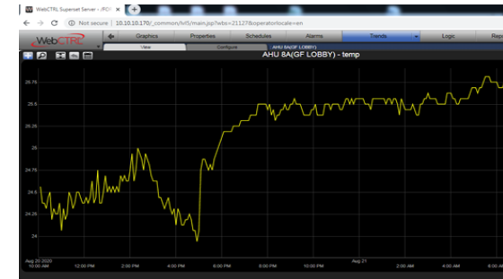
Chiller running optimization done by increase in Temperature set point
